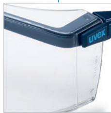
Panorama lens Reliable protective eyewear: The scratch-resistant anti-fog panorama polycarbonate lens with integrated side protectors ensures optimum coverage of the eyes.
